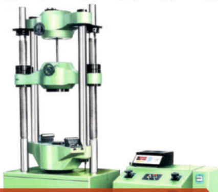
Tensile Testing Machine 20 Tons Cap. Calibration under TUV witness (Cast Speciman from each heat tested mechanically)
